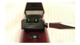
You will have parts left over from the William Fire Sight package: the carrier, the windage screw and the windage adjustment spring. Keep the original blade in a safe place in case you ever need to restore your factory iron sights
