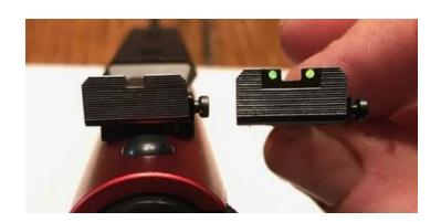
Now install the Williams Fire Sight blade in the factory carrier by inserting the spring, then the blade and then the windage adjustment screw.
