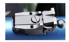
The earlier version of the sight manufactured before July 2018 factory rear sight has only two pieces: the dovetail and the carrier containing the blade. There is only only screw hole in the dovetail and the elevation screw in the carrier.
